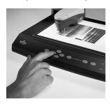
Using the SpectroScan T field command cursor keys (36) , position the measuring device so that the positioning device grid (30) entirely covers the 1st measurement field completely. To check positioning, the Spectrolino may be lowered onto the measuring surface and then raised by means of the Up/Down key. The coordinates of the 1st measurement field are transferred to the software when the Enter key is pressed. To enter the readings for the 2nd and 3rd fields, proceed as described above.
