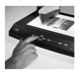
Using the SpectroScan field command cursor keys (36), position the measuring device so that the positioning device grid (30) entirely covers the 1st measurement field completely. To check positioning, the Spectrolino may be lowered onto the measuring surface and then raised by means of the Up/Down key. The coordinates of the 1st measurement field are transferred to the software when the Enter key is pressed. To enter the readings for the 2nd and 3rd fields, proceed as described above.
