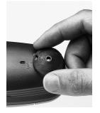
To substitute a filter attached to the aperture, turn the filter tube in a counter clockwise direction until the point of the arrow aligns with the arrow on the instrument. In this position, the filter may be easily removed. To attach new filter, align with the reference arrows and turn clockwise to the end of the mark. This is the only correct position for the filter.
